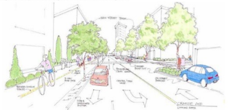
Figure 29. Proposed N. Orange Avenue cross-section looking north.
